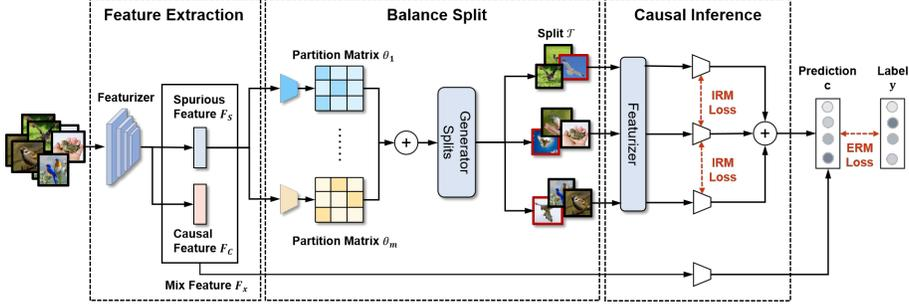
**Fig. 2.** Schematic diagram of the BP-Causal algorithm: the feature extraction module extracts features for subsequent computation; the balance split module divides the dataset into subsets with different environments in a balanced manner; the causal inference module uses IRM Loss and ERM Loss to constrain at the same time, training the ability to extract invariant features for prediction from different environments.
